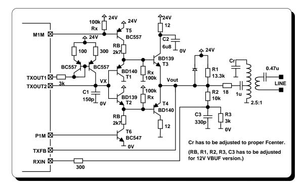
In receive-mode, when the bias-currents are turned off, the base of the two output-transistors are forced by resistors of 100k (Rx) to 0V and Vbuf respectively to guarantee high impedance of the buffer. The current of the pins TxOut1,2 is 0 (VX is floating). Since the receiver-AGC is reacting on signal levels at the RXBPF-filter output, high outband noise-components could give clipping in the first stages of the receiver path. To avoid this, an attenuation of 16dB with R2, R3, C3 is realized.
