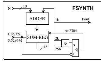
The SC-CLK is defined to be 16 times the center-frequency of the bandpass filters. For generating the FSK or MIXERfrequency, Fsynth gets divided by 16
