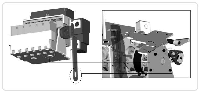
2) Install ON/OFF BUTTON LOCK to the holes of Front base by tightening 2 bolts as shown in figure below.
