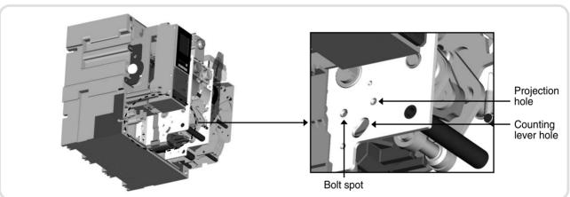
2) Insert the projections of counter to the bottom part of SIDE PLATE of mechanism and put counting lever into counting lever hole.
