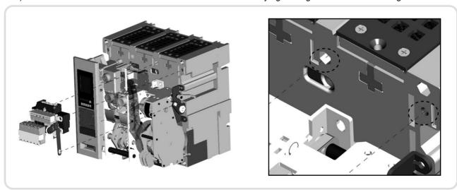
3) Installation method is same for low/high capacity of Aux. contact.
