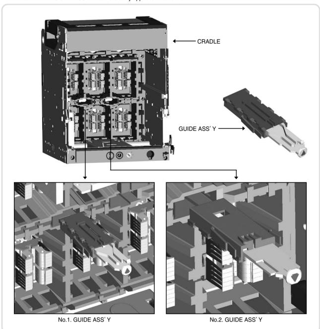
2) Arrange two shutter plates facing each other in the assembly process.
