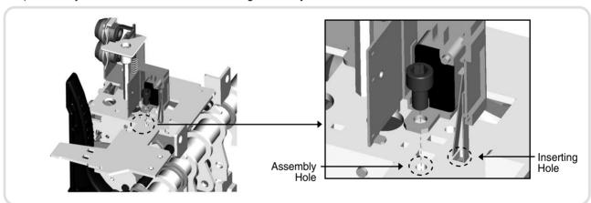
2) Tighten with M4 bolt by using wrench.
