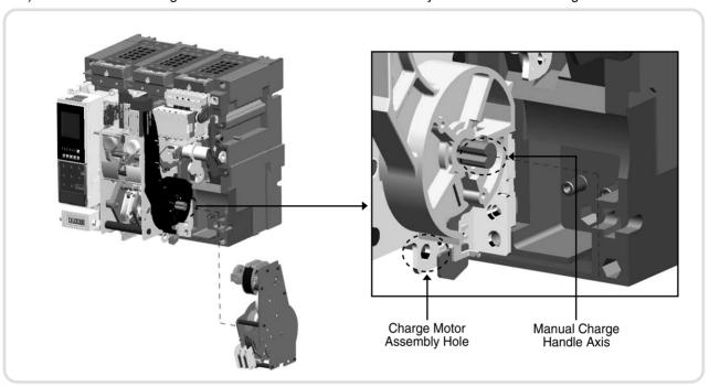
3) Tighten with M6 bolt after fitting the bottom of charge motor into the bottom of mechanism.
