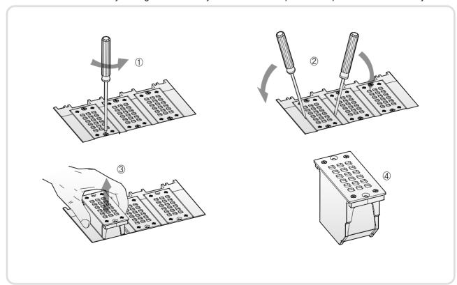
Fig. 7. Separate procedure of Arc chamber
