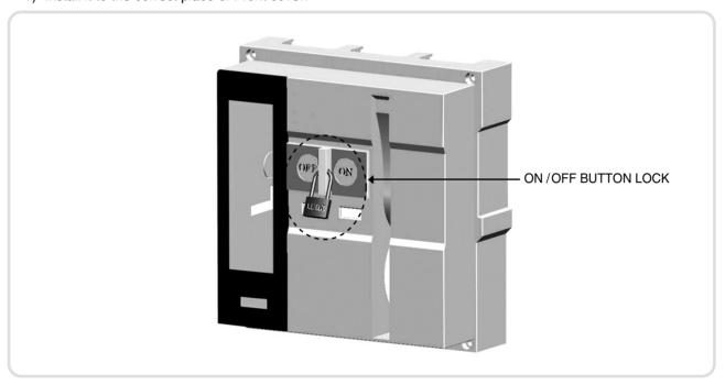
2) Install ON / OFF BUTTON LOCK by using two bolt screws to pass through the holes on inside Front cover as shown in figure above.
