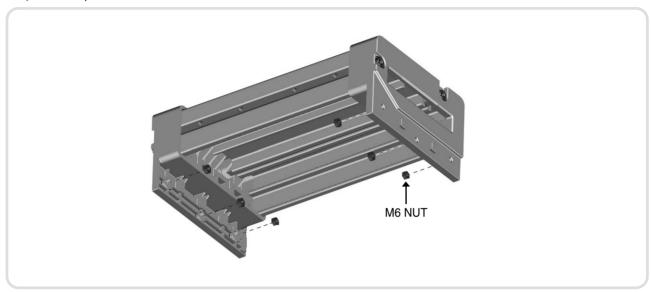
2) Put 6pcs of M6 Bolt into holes of Arc cover and both Side plates and then tighten them.
