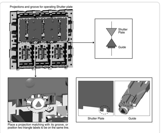
6) The following shows the finished installation of safety shutter to cradle. However, apply the same procedure for installation of safety shutter for bottom.
