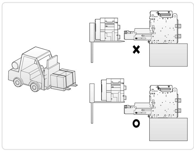
Fig 1. Lifting by forklift
