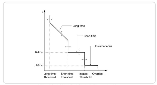
Picture1. Low Voltage Circuit Breaker's Characteristic Curve
