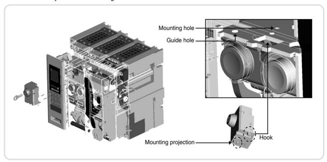
2) Finish the installation by tightening the corresponding screws.
