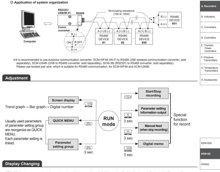
KRN100 displays measuring value as trend graph, bar graph, and digital number display (1-channel, 8-channel, 12-channel). You can select one by the key.
