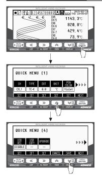
Press the ENTER key once in RUN mode and it enters to QUICK MENU. QUICK MENU consists of usually used parameters for quickly parameter setting.
