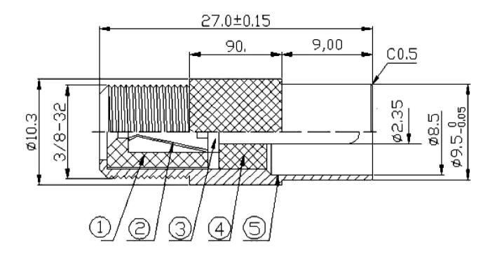
Temp.range  $-65 \sim +250$ Impedance  $75 \Omega$ Frequency Range  $0 \sim 6 \text{GHz}$ Working Voltage 335 V max
